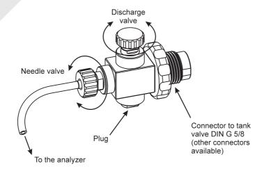
The analyzer switches into the helium and oxygen measuring mode upon activation, so there is no need for you to set up anything. Open the valve on the bottle to let the gas flow in. The gas composition is displayed after approximately 5-10 seconds. If the pressure inside the bottle is distinctly lower than 200 bars, the gas flow through the sampler will be slower and the measuring result will take somewhat longer to determine.
